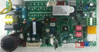
**Solution:** Check the connecter of sensor and slot (CN6, CN6-1, CN6-2), if loose or not plugged in, please connect again.
