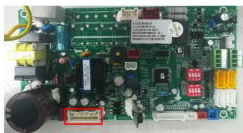
Solution: Check the connecter of indoor motor and slot (CN3) and (CN4), if loose or not plugged in, please connect again.
