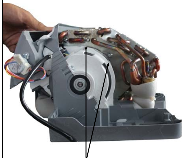
Two screws at the base bearing side
