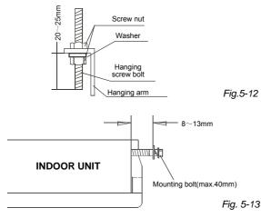
· Hang the unit on the hanging arm by sliding backward. Securely tighten the mounting bolts on both sides. (Refer to Fig. 5-14) (some of the models 60 do not do this)
