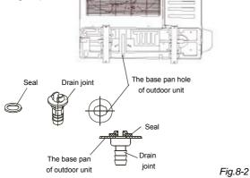
Outdoor unit is equiped with a drain piping. Its position is shown figure below
