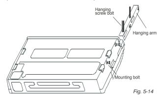
For some of the models 60 please securely tighten the mounting bolts on both sides. (Refer to Fig5-15).
