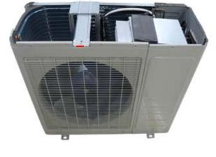
Fan ass'y How to remove the fan Electronic control box Fan ass'y. 1) After remove the panel plate following procedure 1, remove the hex nut fixing the fan and then remove the fan. Two reactors Compressor and liquid-gas separator Nut fixing the fan 2) Remove the one fixing screw. Unfix the hooks and then open the electronic control box cover.
