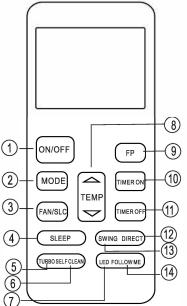
and then be off for 2 seconds by turns. Press ON/OFF,SLEEP, FP, MODE, FAN SPEED,UP, DOWN buttonwhile operating will cancel the freeze protection function.
