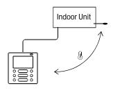
When the Follow me function indication pears, the room temperature is detected at the wire controller.
