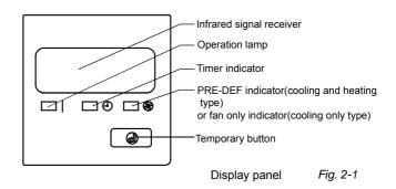
This function is used to operate the unit temporarily in case you misplace the remote controller or its batteries are exhausted. Two modes including AUTO and FORCED COOL can be selected through the TEMPORARY BUTTON on the display panel. Once you push this button, the air conditioner will run in such order: AUTO, FORCED COOL,(COOLING TEST HEATING TEST,)OFF, and back to AUTO.
