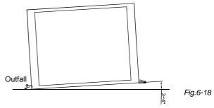
NOTE: Make sure 3-4 degree of angel is kept between the unit and the floor when the unit is installed in the low temperauture and humid environment.
