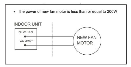
■ Fig.10-10 (the figure is for the unit with the new fan function)
